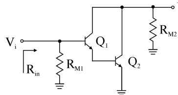
$$R_{in} = R_{M1} // [ r_{\pi 1} + (1 + \beta_1)r_{\pi 2} ] \\ = 15.02 // [ 77.78 + (1 + 100) \times 0.77 ] \\ = 13.7k\Omega$$
