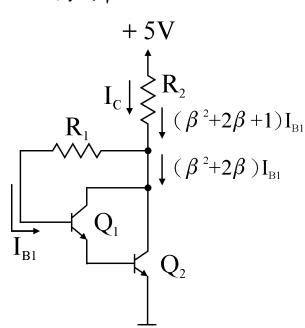
$$\begin{aligned} I_{B1} &= \frac{5 - 0.7 - 0.7}{R_1 + (\beta^2 + 2\beta + 1)R_2} \\ &= \frac{5 - 0.7 - 0.7}{1000 + (100^2 + 200 + 1) \cdot 1} = 3.214 \times 10^{-4} \text{ mA} \\ I_C &= (\beta^2 + 2\beta + 1)I_{B1} \\ &= (100^2 + 200 + 1) \times 3.214 \times 10^{-3} = 3.28 \text{ mA} \end{aligned}$$
