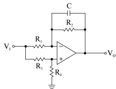
$$\Rightarrow \frac{V_o}{V_i} = -\frac{R_2}{R_1} \cdot \frac{1}{1+SCR_2} + \frac{1+SCR_2 + \frac{R_2}{R_1}}{1+SCR_2} \cdot \frac{\frac{R_2}{R_1}}{1+\frac{R_2}{R_1}}$$
