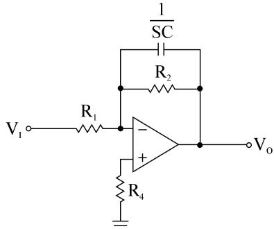
$$T(S) = \frac{V_o(S)}{V_i(S)} = -\frac{\frac{1}{SC}}{R_1} = \frac{-\frac{1}{R_1 C}}{S + \frac{1}{R_2 C}}$$
