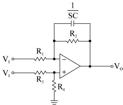
$$V_o = \left[ -\frac{R_2}{R_1} \cdot \frac{1}{1+SCR_2} + \left( 1 + \frac{R_1}{1+SCR_2} \right) \left( \frac{R_4}{R_3 + R_4} \right) \right] V_i$$
