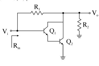
$$\begin{aligned} I_{B2} &= (1 + \beta_1)I_{B1} = (1 + 100) \times 3.214 \times 10^{-4} \text{ m} \\ &= 0.0325 \text{ mA} \\ r_{\pi 1} &= \frac{V_T}{I_{B1}} = \frac{25 \text{ m}}{3.214 \times 10^{-4} \text{ m}} = 77.78 \text{ k}\Omega \\ r_{\pi 2} &= \frac{V_T}{I_{B2}} = \frac{25 \text{ m}}{0.0325 \text{ m}} = 0.77 \text{ k}\Omega \end{aligned}$$
