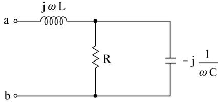
$$Z_{ab} = \frac{R \times (-j \frac{1}{\omega C})}{R - j \frac{1}{\omega C}} + j\omega L = \frac{-jR}{\omega RC - j} + j\omega L = \frac{-jR(\omega RC + j)}{(\omega RC)^2 + 1} + j\omega L$$
