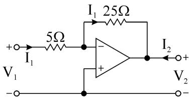
$$V_- = V_+ = 0 \text{ (V)} , I_1 = \frac{V_1}{5} = g_{11}V_1 + g_{12}I_2$$
