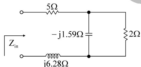
$$\begin{aligned} \therefore \text{等效阻抗 } Z_{in} &= [2 // (-j1.59)] + 5 + j6.28 = 0.7745 - j0.974 + 5 + j6.28 \\ &= 5.7745 + j5.306\text{ (\Omega)} \end{aligned}$$
