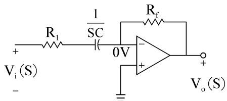
$$\frac{0 - V_i(S)}{R_1 + \frac{1}{SC}} + \frac{0 - V_o(S)}{R_f} = 0$$
