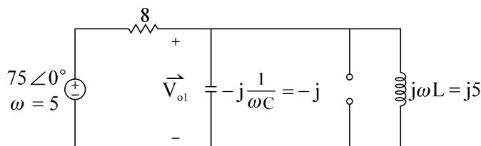
$$\frac{\vec{V}_{o1} - 75\angle 0^\circ}{8} + \frac{\vec{V}_{o1}}{-j} + \frac{\vec{V}_{o1}}{j5} = 0 \Rightarrow \vec{V}_{o1} = 11.58\angle -81.12^\circ$$
