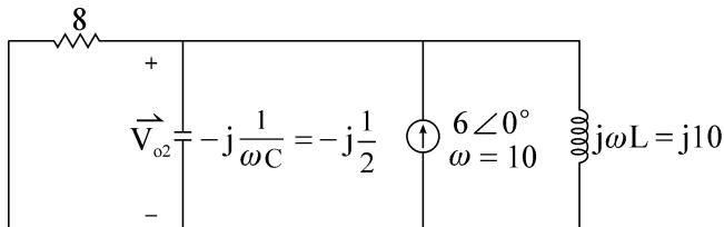
$$\frac{\vec{V}_{o2}}{8} + \frac{\vec{V}_{o2}}{-j\frac{1}{2}} + \frac{\vec{V}_{o2}}{j10} = 6 \angle 0^\circ \Rightarrow \vec{V}_{o2} = 3.151 \angle -86.236^\circ$$
